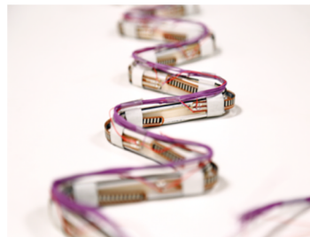
Figure 3: The bendable interface without the fabric cover. Images display the bend sensors on segments of styrene connected through thin wires.
